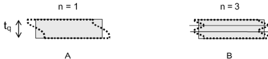
Fig. 2.6: A schematic illustration of thickness-shear mode displacements. In A) the fundamental mode: the thickness of the crystal, t_q , equals half an acoustic wavelength. In B) the third overtone: the thickness of the crystal equals 3/2 acoustic wavelengths.
